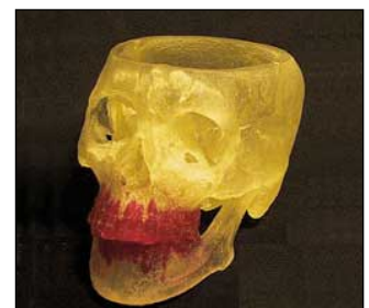
Figure 5: Anatomical model of a skull made by coloured stereolithography.
