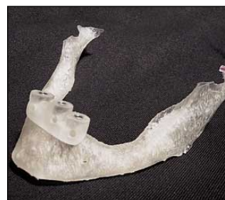
Figure 4: SurgiCase drill guide located on an anatomical model of a mandible, showing the exact fit (courtesy of Dr. A. Sethi).
